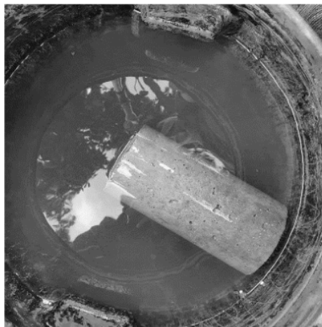
Figure 6 APPB concrete in floating condition
