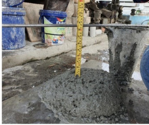
Figure 3 Slump test measurement
