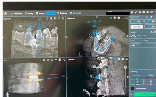
FIGURE 2 ExcelsiusGPS software screw planning includes entry points, trajectories, screw length, and width.
