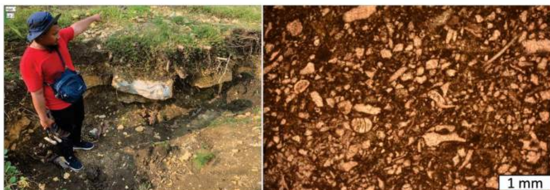
Fig. 3. Appearance of limestone with Clastic facies Packstone LP 2 (left) and thin section of Packstone limestone (right)
