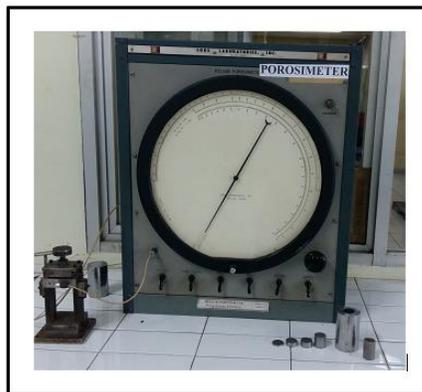
Gambar 3.7 *Helium Porosimeter*
