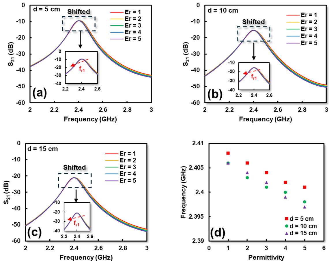
Figure. 2 Simulation detection of tan delta with range of  $d = 5 \text{ cm} - 15 \text{ cm}$  using proposed sensor; (a)  $d = 5 \text{ cm}$ , (b)  $d = 10 \text{ cm}$ , (c)  $d = 15 \text{ cm}$ , (d) correlation between distance with resonance frequency and permittivity of samples, (e) correlation between distance and  $S_{21}$
