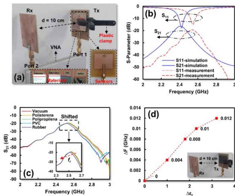
Figure 5. Measurement of proposed sensor; (a) setup for detection using tagging antenna sensor, (b) simulation and measurement result, (c) response of frequency with permittivity changes, (d)  $\Delta F$  of proposed sensor.
