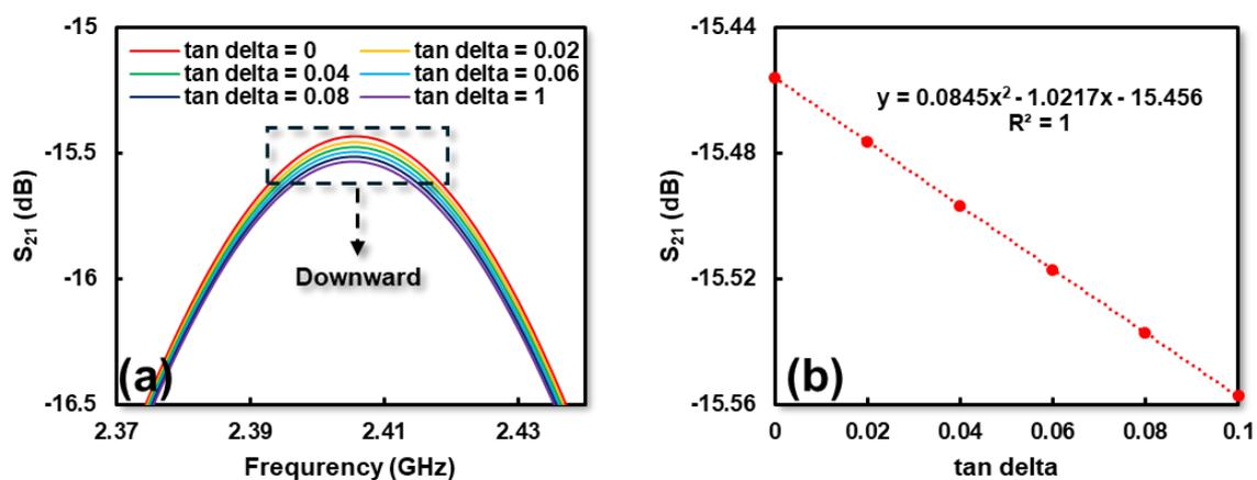
**Fig.1** Simulation detection of tan delta with range of 0 – 0.1 using proposed sensor; (a) correlation resonance frequency with tan delta, (b) correlation between  $S_{21}$  and tan delta
