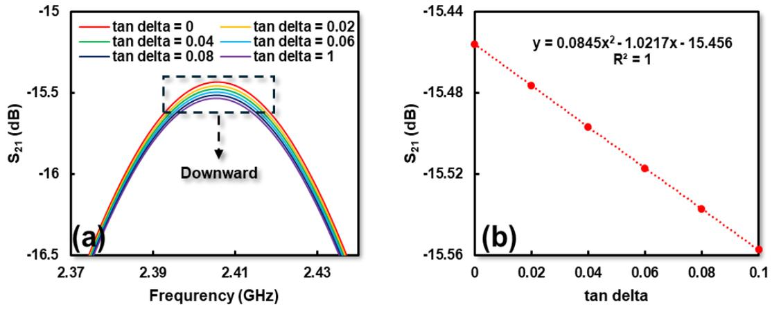
Figure 5. Simulation detection of  $\tan \delta$  with range of 0 – 0.1 using proposed sensor; (a) correlation resonance frequency with  $\tan \delta$ , (b) correlation between  $S_{21}$  and  $\tan \delta$
