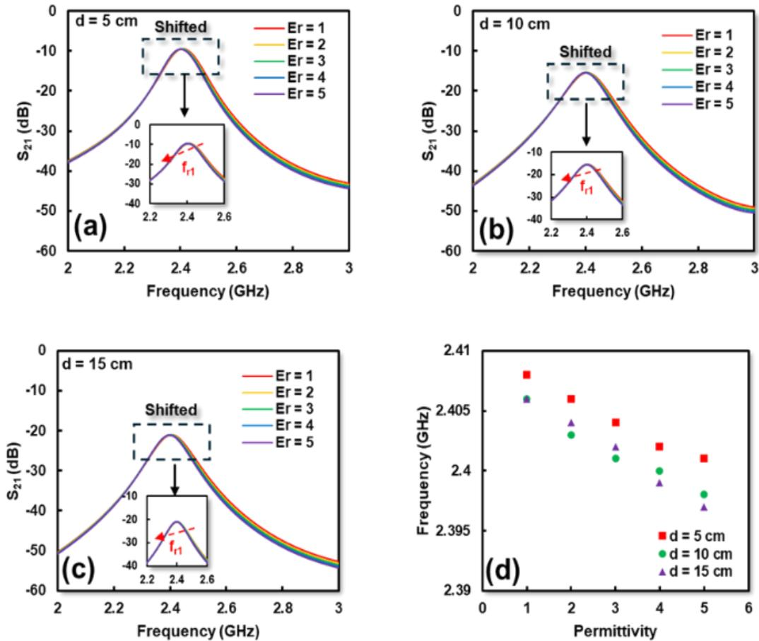
Figure 6. Simulation detection of  $\tan \delta$  with range of  $d = 5$  cm – 15 cm using proposed sensor; (a)  $d = 5$  cm, (b)  $d = 10$  cm, (c)  $d = 15$  cm, (d) correlation between distance with resonance frequency and permittivity of samples, (e) correlation between distance and  $S_{21}$
