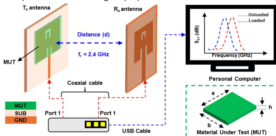
**Figure 1.** Proposed scenario for permittivity detection based on tagging antenna sensor
