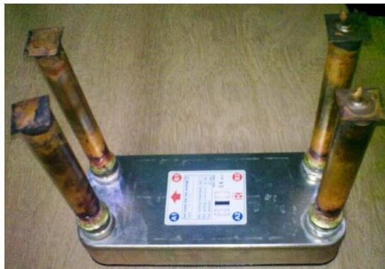
Gambar 3.15. *Plate Heat Exchanger*
