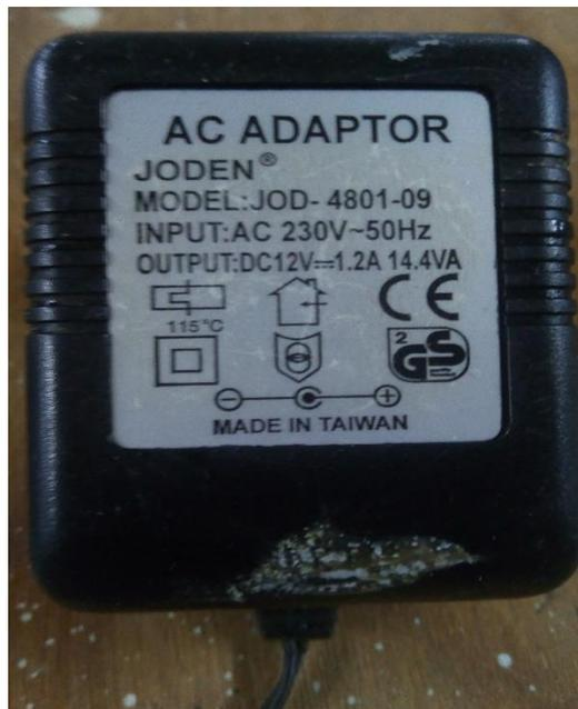
Gambar 3.6. *Power Supply Pressure Transmitter*
