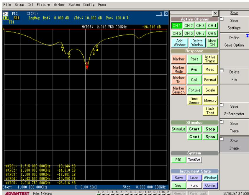
**Gambar 3.25** Hasil Pengukuran *Return Loss*
