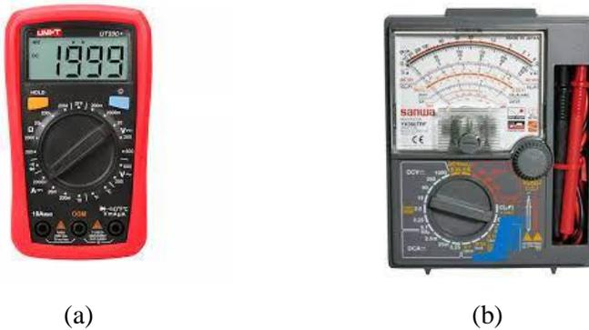
**Gambar 3.3** Multimeter; (a) digital, (b) analog
