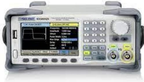
**Gambar 6.8** Digital Function Generator.
