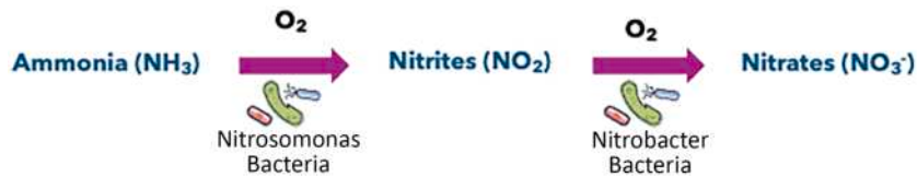
Figure 8.8 The nitrification process in freshwater.
