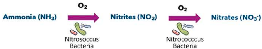
Figure 8.9 The nitrification process in saltwater.
