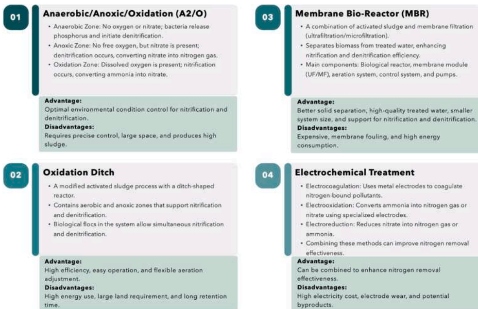
Figure 23.3 Advanced nitrogen removal technologies for wastewater treatment.
