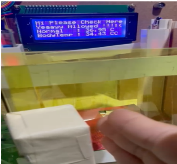
Figure 11: Body Temperature Measurement Using MLX 90614 Sensor
