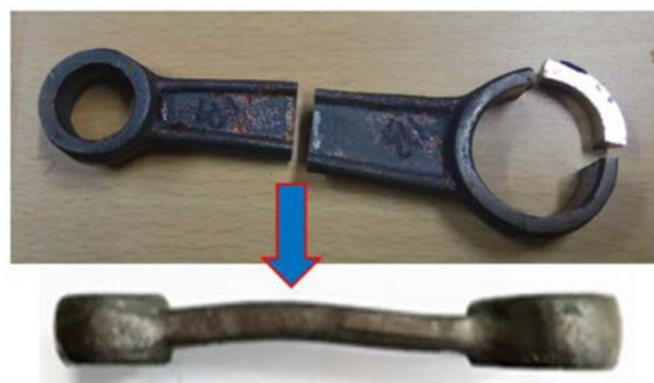
Fig. 5. Position for metallography examination.
