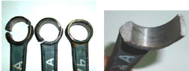
Figure 4. Break point during tensile test.
