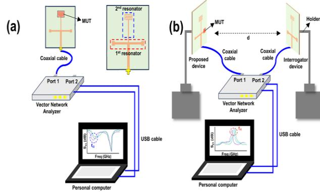
**Fig. 1.** Scenario of permittivity detection using proposed sensor; (a) scenario (1) for contactless detection using an interrogator antenna, (b) scenario (2) for contact detection
