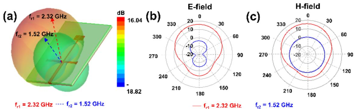
**Fig.3** (a) Radiation pattern of proposed resonator at  $f_{r1} = 2.32$  GHz and  $f_{r2} = 1.52$  GHz, (b) E-field at  $f_{r1} = 2.32$  GHz and  $f_{r2} = 1.52$  GHz, (c) H-field at  $f_{r1} = 2.32$  GHz and  $f_{r2} = 1.52$  GHz.
