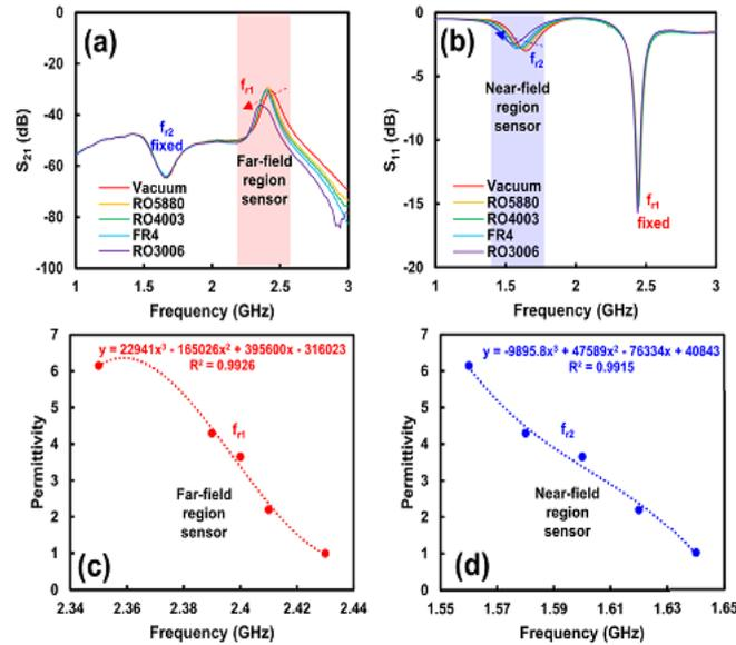
**Fig. 7.** Permittivity detection using proposed sensor, (a) contactless detection with  $d = 10$  cm, (b) contact detection, (c) polynomial equation for contactless detection, (d) polynomial equation for contact detection.
