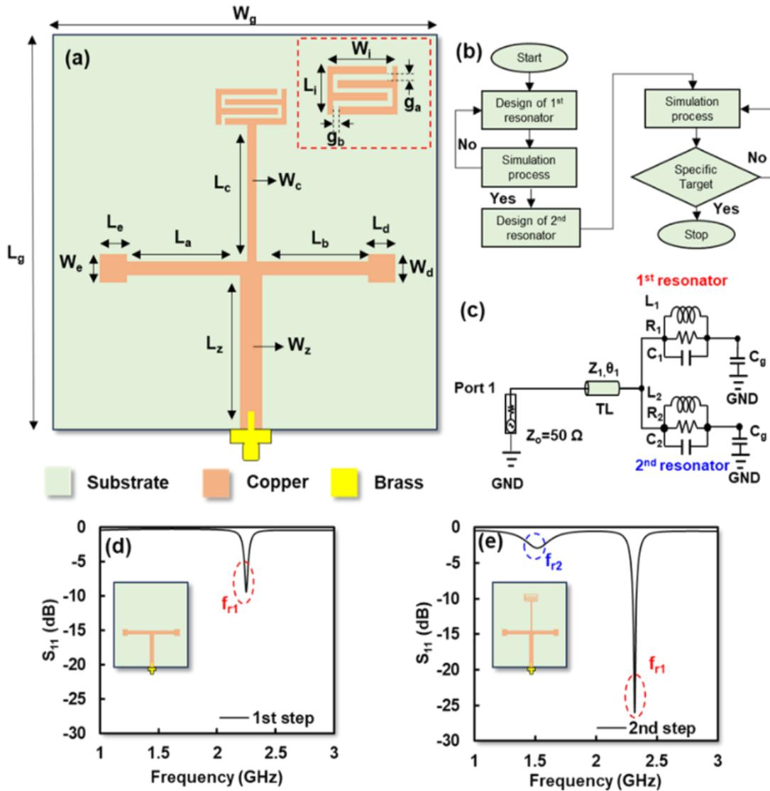
**Fig. 4.** (a) Structure of T-shaped resonator, (b) flowchart of design process, (c) equivalent circuit, (d) 1<sup>st</sup> step model, (e) 2<sup>nd</sup> step model.
