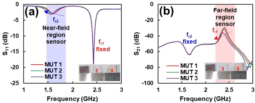
**Fig 8.** (a) Contact detection for unknown MUT, (b) long-range detection for unknown MUT
