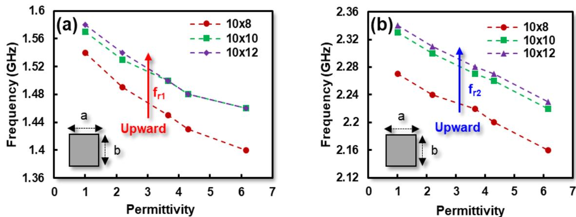
**Fig.1** Response of resonance frequency based on different sample dimensions; (a) long-range detection, (b) contact detection
