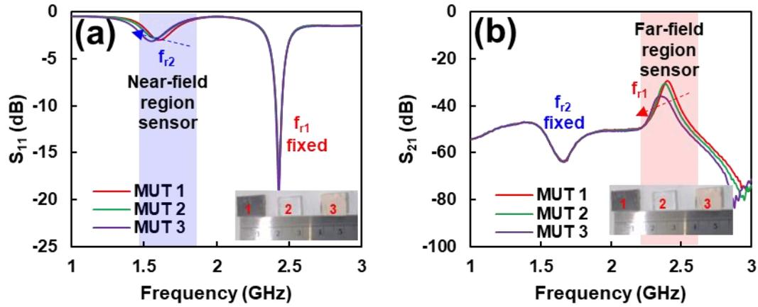
**Fig 1.** (a) Contact detection for unknown MUT, (b) long-range detection for unknown MUT
