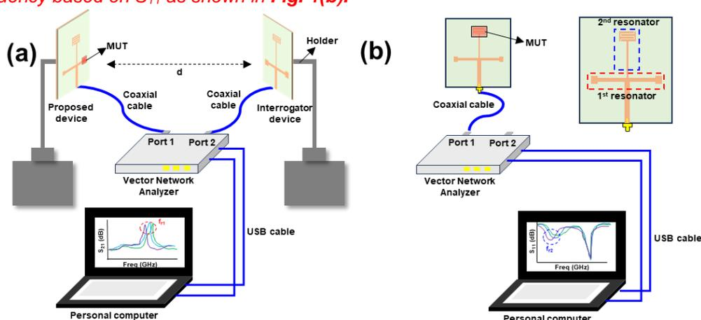
**Fig. 1.** Scenario of permittivity detection using proposed sensor; (a) scenario (1) for long-distance detection using an interrogator antenna, (b) scenario (2) for contact detection
