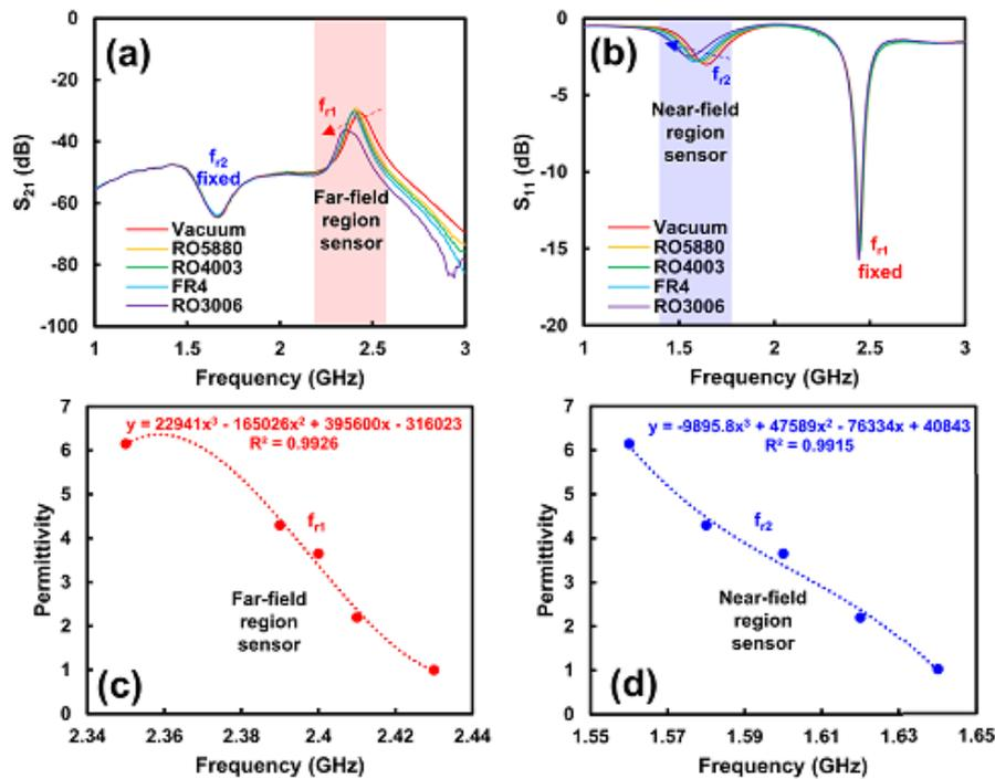
**Fig. 7.** Permittivity detection using proposed sensor, (a) contactless detection with  $d = 10$  cm, (b) contact detection, (c) polynomial equation for contactless detection, (d) polynomial equation for contact detection.
