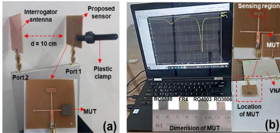
**Fig. 6.** Measurement setup; (a) long-distance detection using scenario (1), (b) contact detection using scenario (2).
