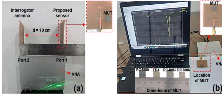
**Fig. 6.** Measurement setup; (a) contactless detection using scenario (1), (b) contact detection using scenario (2).
