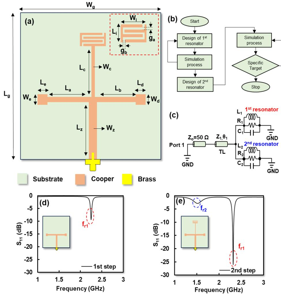
**Fig. 4.** (a) Structure of T-shaped resonator, (b) flowchart of design process, (c) equivalent circuit, (d) 1<sup>st</sup> step, (e) 2<sup>nd</sup> step.
