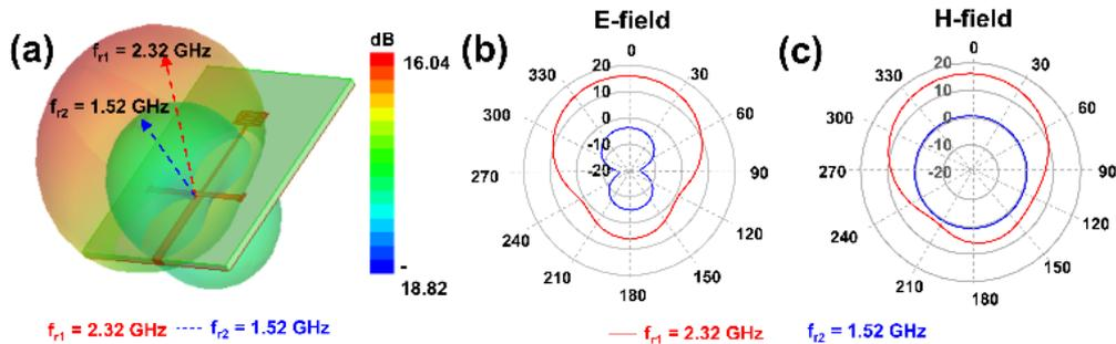
**Fig.3** (a) Radiation pattern of proposed resonator at  $f_{r1} = 2.32$  GHz and  $f_{r2} = 1.52$  GHz, (b) E-field at  $f_{r1} = 2.32$  GHz and  $f_{r2} = 1.52$  GHz, (c) H-field at  $f_{r1} = 2.32$  GHz and  $f_{r2} = 1.52$  GHz.
