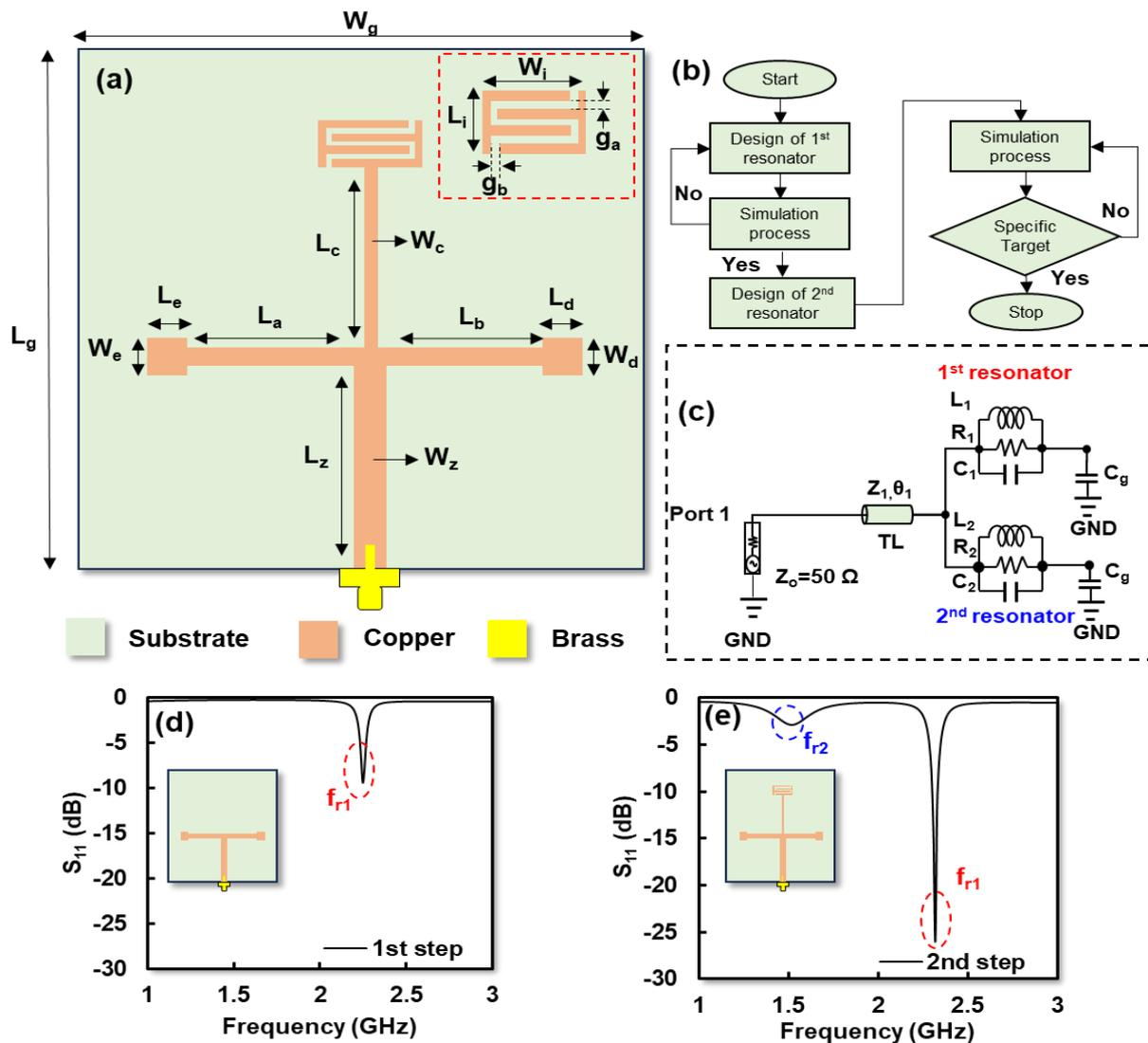
Fig. 1. (a) Structure of T-shaped resonator, (b) flowchart of design process, (c) equivalent circuit, (d) 1<sup>st</sup> step model, (e) 2<sup>nd</sup> step model.
