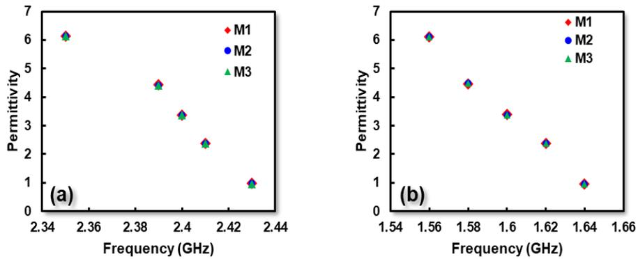
**Fig.3** Repeatability of measurement using proposed sensor; (a) long-range detection, (b) contact detection
