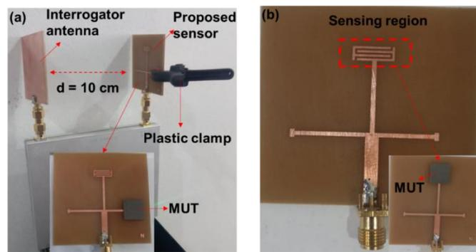
Fig 1. Placement of MUT; (a) for contactless detection, (b) for contact detection
