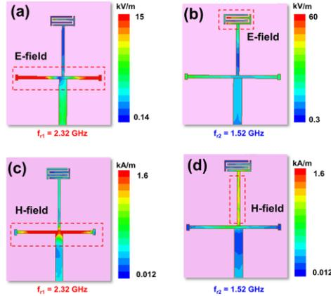
**Fig.2** E-field and H-field concentration; (a) E-field at  $f_{r1} = 2.32$  GHz, (b) E-field at  $f_{r2} = 1.52$  GHz, (c) H-field at  $f_{r1} = 2.32$  GHz, (d) H-field at  $f_{r2} = 1.52$  GHz.
