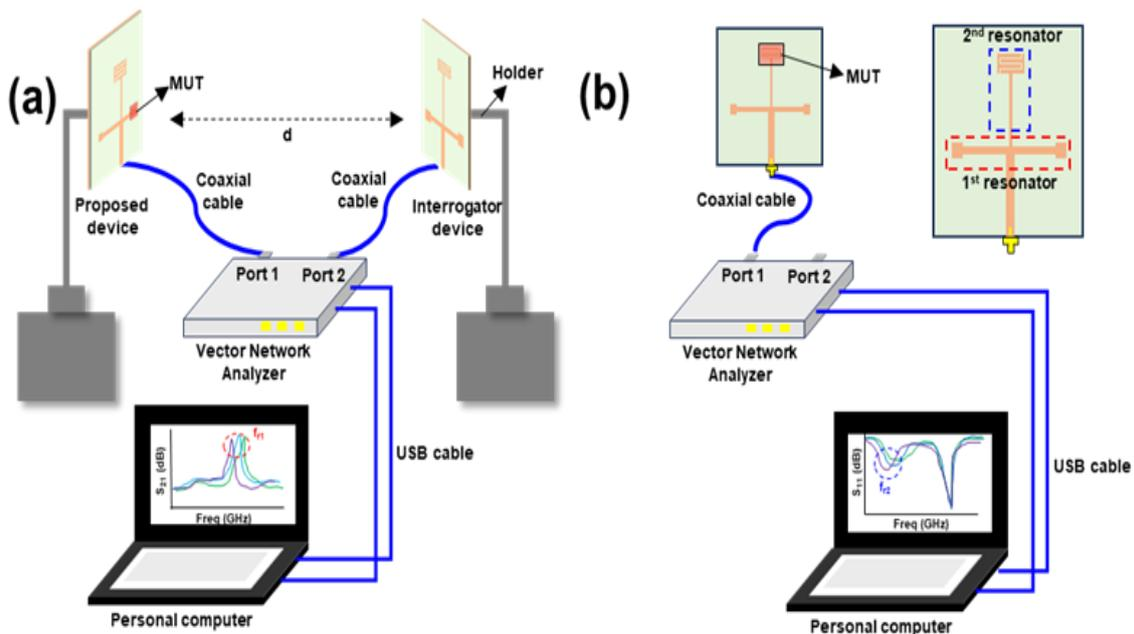
**Fig. 1.** Scenario of permittivity detection using proposed sensor; (a) scenario (1) for long-distance detection using an interrogator antenna, (b) scenario (2) for contact detection
