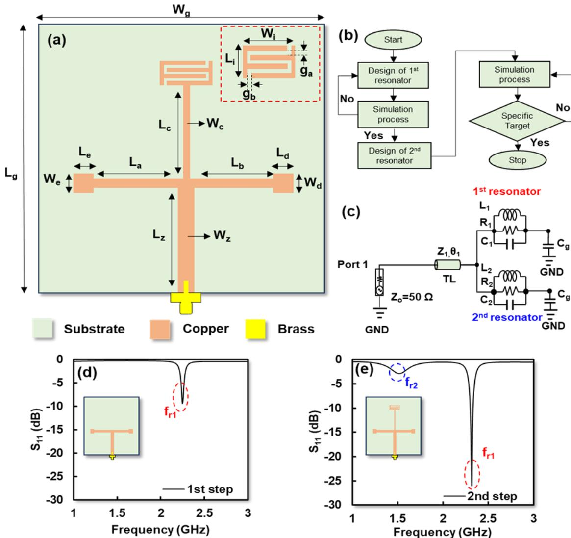
**Fig. 4.** (a) Structure of T-shaped resonator, (b) flowchart of design process, (c) equivalent circuit, (d) 1<sup>st</sup> step model, (e) 2<sup>nd</sup> step model.
