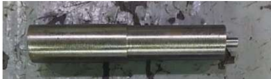
Figure 3. Tool shoulder with 7 mm pin (after turning).
