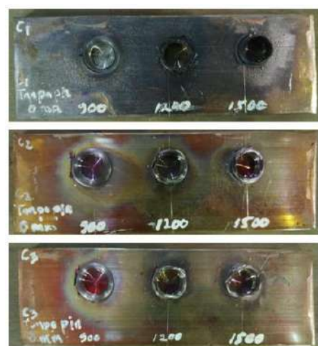
Figure 20. Samples C1, C2, and C3 top view of FSSW welding without pin (0 mm) welding depth of 2 mm.
