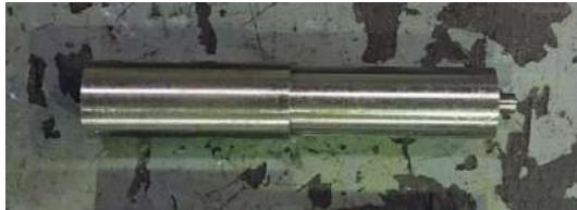
Figure 4. Tool shoulder with 5 mm pin (after turning).
