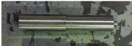
Figure 4. Tool shoulder with 5 mm pin (after turning).
