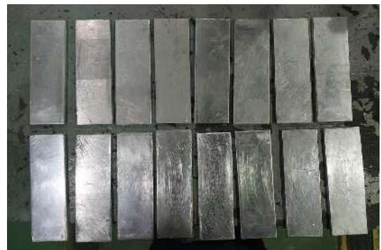
Figure 8. Aluminum material 150x50x5 mm.
