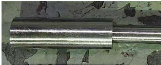
Figure 5. Tool shoulder without pin (after turning).
