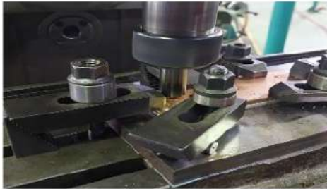
Figure 12. Clamping Kit used in the FSSW process.
