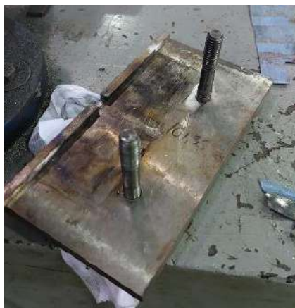
Figure 13. Base Kit used in the FSW process.
