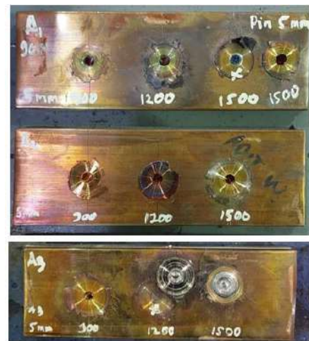
Figure 18. Samples A1, A2, and A3 top view of FSSW welding results with 5 mm pin 5.1 mm welding depth.
