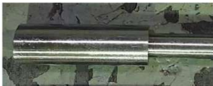
Figure 5. Tool shoulder without pin (after turning).
