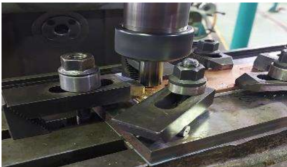
Figure 12. Clamping Kit used in the FSW process.
