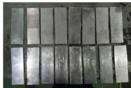
Figure 8. Aluminum material 150x50x5 mm.
