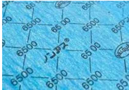
Figure 14. Gaskets used in the FSW process.
