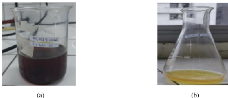
Figure 2. Used cooking oil before being purified (a) and used cooking oil after being purified (b)
