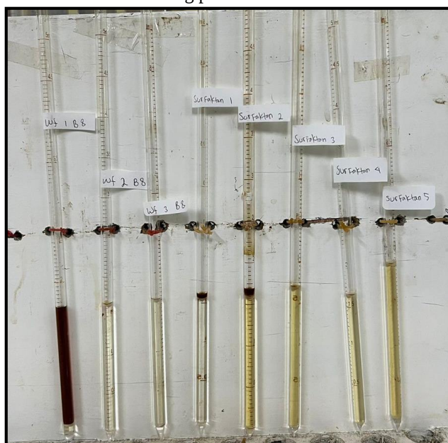
Figure 5. Oil recovery during ABS surfactant coreflood
