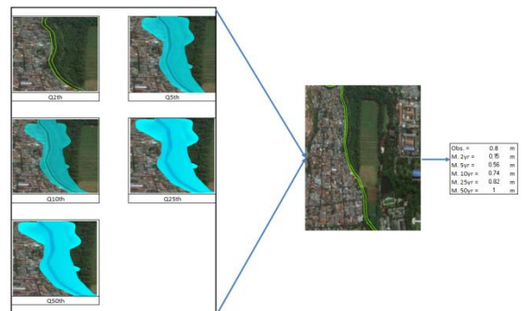
Figure 7. Comparison between observed and modeling inundation in South of Jakarta area: a) modeled, b) observed
