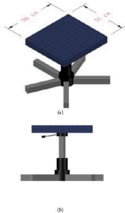
Fig. 7. Adjustable workbench for welders: (a) isometric view and (b) front view.
