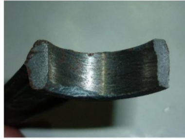
Figure 5. Break point during tensile test.
