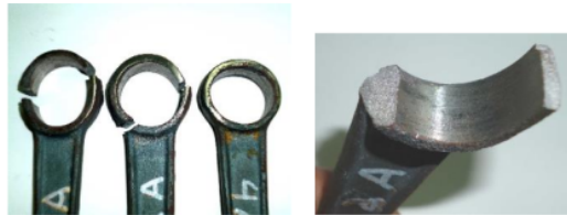
Figure 4. Break point during tensile test.
