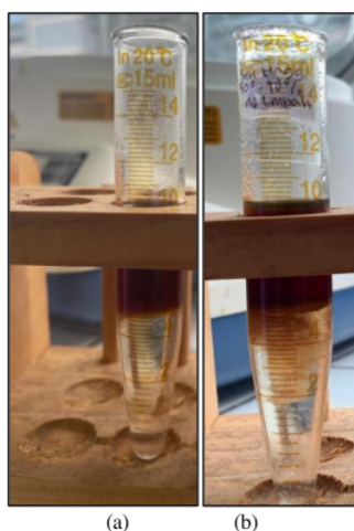
Figure 3. Demulsification Test at 70% Salinity Water a). Without Diaper Waste b). With Diaper Waste
