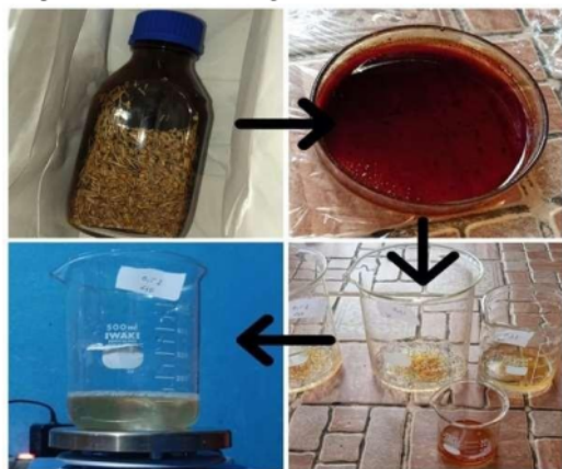
Fig. 1. The process of lemongrass leaves extraction by maceration method and encapsulation with chitosan by ionic gelation method.
