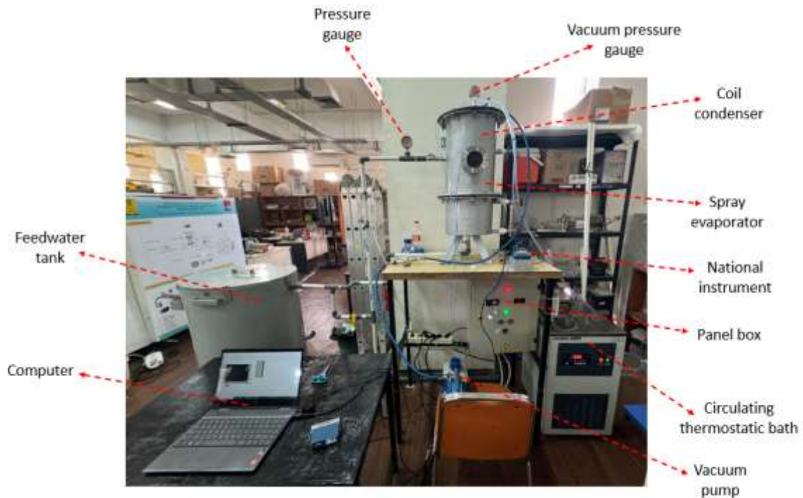
Gambar 3.2 Susunan Eksperimen Direct Spray Evaporator dan Cooling Coil Condenser Skala Laboratorium
