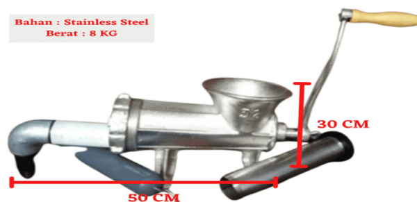
Gambar 6. Mesin Pelinting Dodol
