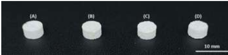
Figure 1. Composite blocks containing 70 % Sigma-Aldrich \beta TCP Control with 30 % PAA (A), 60 % \beta TCP from green mussel shells with 40 % PAA (B), 65 % \beta TCP from green mussel shells with 35 % PAA (C), and 70 % \beta TCP from green mussel shells with 30 % PAA composite blocks (D).
