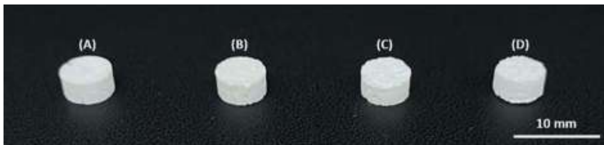
Figure 1. Composite blocks containing (A) 70% Sigma-Aldrich beta-tricalcium phosphate ( \beta -TCP) control with 30% polyacrylic acid (PAA) (SA-P), (B) 60% green mussel shell-derived \beta -TCP with 40% PAA (B60-P40), (C) 65% green mussel shell-derived \beta -TCP with 35% PAA (B65-P35), and (D) 70% green mussel shell-derived \beta -TCP with 30% PAA (B70-B30).
