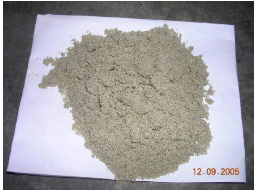
Figure 3. 3: 300-425 \mu m Sand Particles
