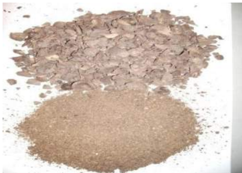
Figure 3.12 Palm shell fuel (before and after grinding)
