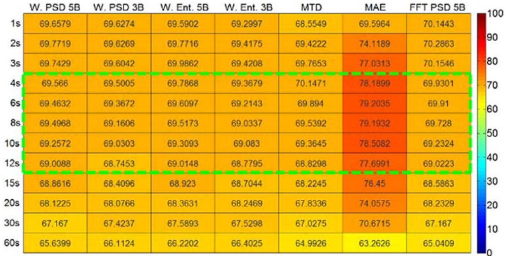
Figure 17.8 OWS color graph. The numbers in the graph depict the weighted average accuracy of four emotion planes for every seven features. For each of the seven features, the color heatmap displays various levels of accuracy yielded by window size between 1 and 60 s, with darker colors indicating higher accuracy. The best window can be found by looking at the graph. OWS, Optimal window selection.
