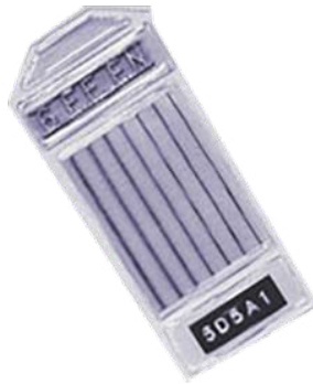
Gambar 7.7 Contoh IQI (ndt-instrument.com)
