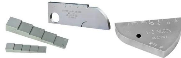
Gambar 4.21. Contoh Block Standar
