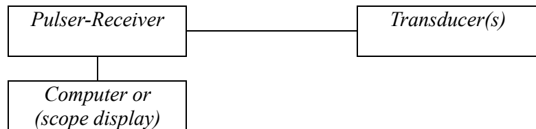
Gambar 4.6 Koneksitas Antara Unit Pulser-Receiver; Transducer' Computer Or (Scope Display)
