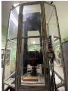
Gambar 3. 94 Universal Testing Machine (UTM) 1000 kN
