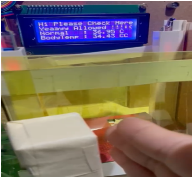
Figure 11: Body Temperature Measurement Using MLX 90614 Sensor
