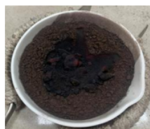
Fig. 2. Galena concentrate in powder form after roasting process
