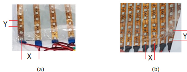
Figure 4: Comparison of LED spacing, (a) Before (unwanted), (b) After (as desired)
