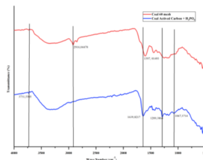
Figure 3. Fourier Transform Infrared Spectroscopy (FTIR) of coal activated carbon using phosphoric acid (AC3)
