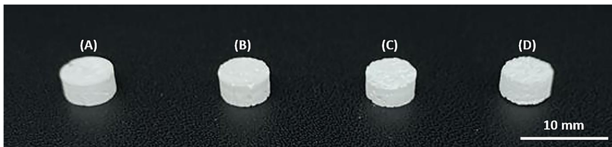
Figure 1. Composite blocks containing (A) 70% Sigma-Aldrich beta-tricalcium phosphate ( \beta -TCP) control with 30% polyacrylic acid (PAA) (SA-P), (B) 60% green mussel shell-derived \beta -TCP with 40% PAA (B60-P40), (C) 65% green mussel shell-derived \beta -TCP with 35% PAA (B65-P35), and (D) 70% green mussel shell-derived \beta -TCP with 30% PAA (B70-P30).
