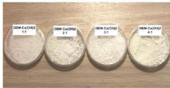
**Figure 1.** DBM-Ca(OH)<sub>2</sub> prepared for four different weight ratios: 1:1, 2:1, 3:1, and 4:1.
