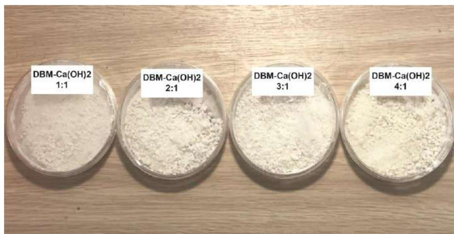
**Figure 1.** DBM-Ca(OH)<sub>2</sub> prepared to four different weight ratios: 1:1, 2:1, 3:1, and 4:1.
