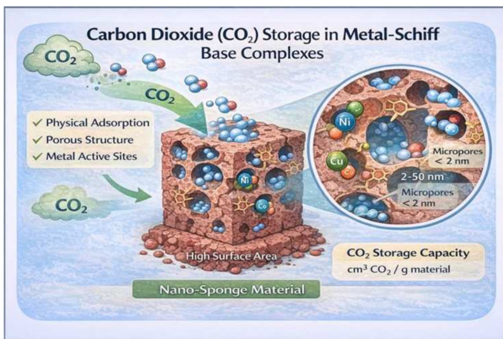
Fig. 3. Schematic representation of \text{CO}_2 storage in porous metal-Schiff base complexes, illustrating physical adsorption of \text{CO}_2 within micro- and mesopores, adsorption on internal pore surfaces, and weak interactions with metal active sites (Ni, Cu, and Co), highlighting their nano-sponge behavior and high surface area.
