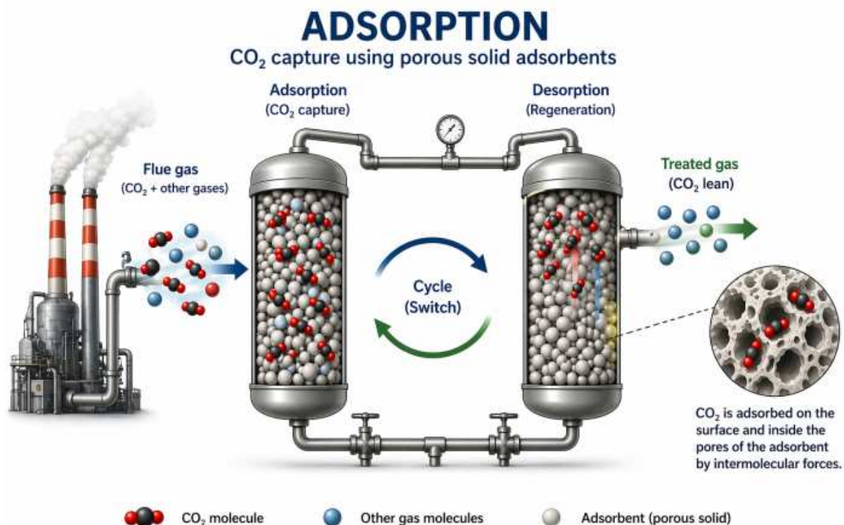
Fig. 3. Schematic illustration of \text{CO}_2 capture by adsorption using porous solid materials, showing adsorption–desorption cycles for efficient gas separation.
