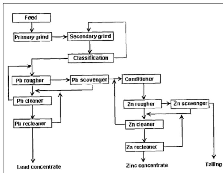
Figure 2. Flowchart of zinc and lead recovery from mineral ore <sup>[10]</sup>
