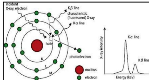
Figure 4. Conceptual theory of X-Ray Fluorescence (XRF) <sup>[13]</sup>
