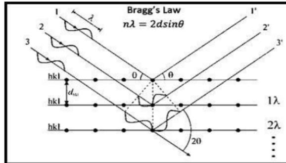
Figure 3. Conceptual theory of X-Ray Diffraction (XRD) with Bragg's Law <sup>[12]</sup>
