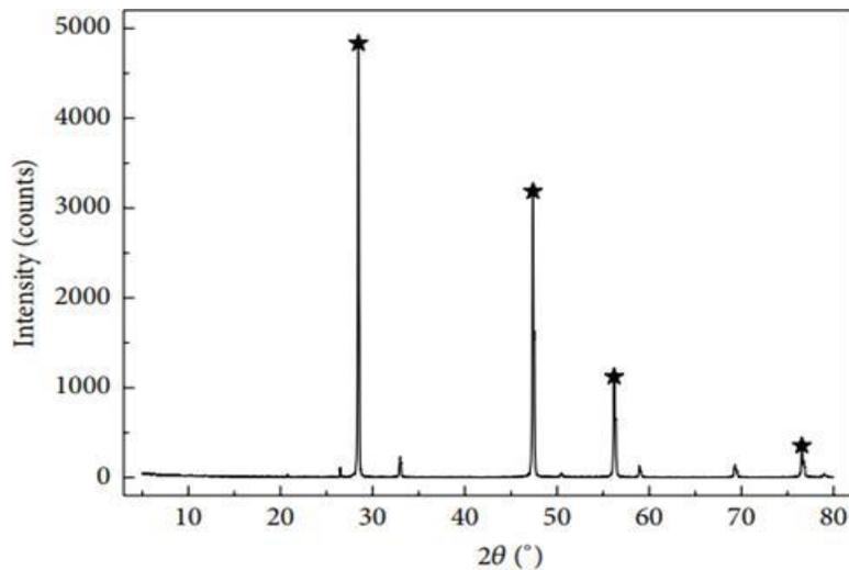
**Figure 6.** XRD pattern of standard sphalerite sample <sup>[15]</sup>
