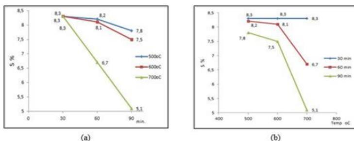
**Figure 11.** Data XRF for S (%) based on (a) varied roasting time and (b) varied roasting temperature.
