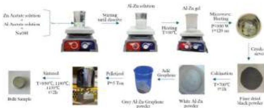
Fig. 1 Schematic illustration of synthesis of Al-doped ZnO/graphene powder by a microwave-assisted sol-gel method
