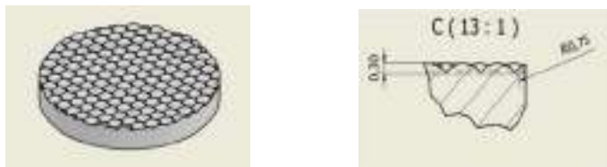
Fig. 1 Detail drawing of micro dimple's substrate
