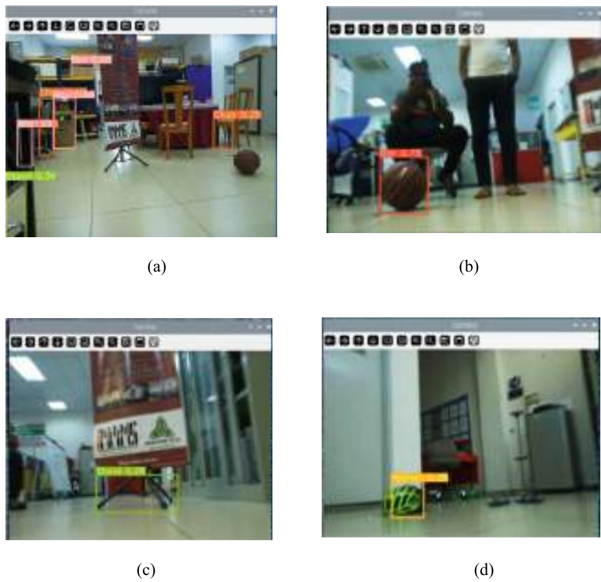
Fig. 5 Obstacles detected by mobile robot: a lab environment objects, b ball, c stand, d helmet
