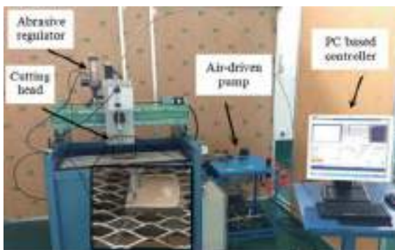
Fig. 3 The self-developed CNC AWJ machine [13]
