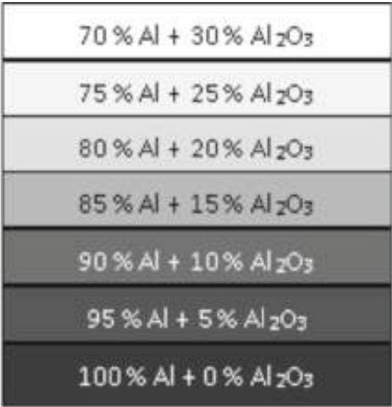
Fig. 1 Percentage compositions for each layer of seven-layered Al-Al 2 O 3 graded composite
