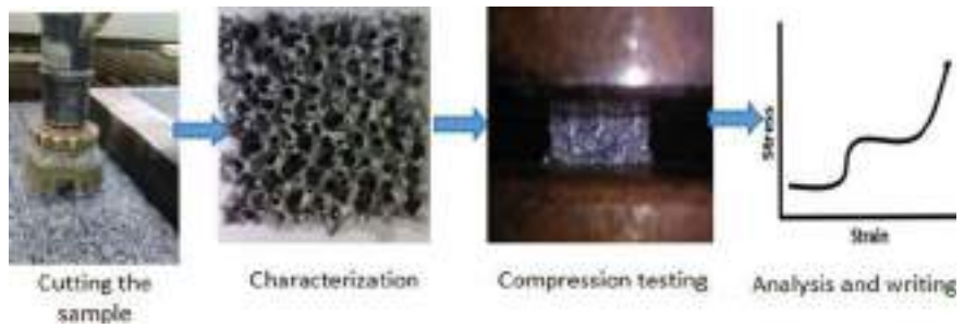
Fig. 4 The flow of the experimental work
