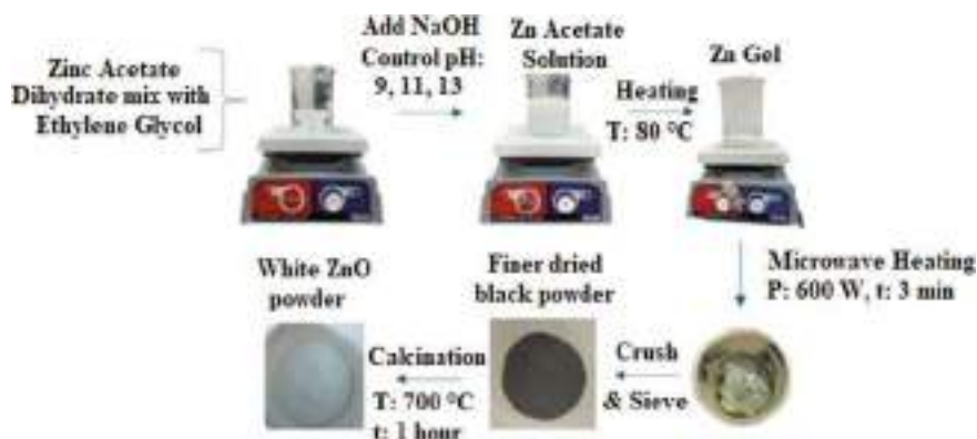
Fig. 1 Schematic illustration of synthesis of ZnO nanoparticles by a microwave-assisted sol-gel method at microwave heating (Power: 600 W time: 3 min)
