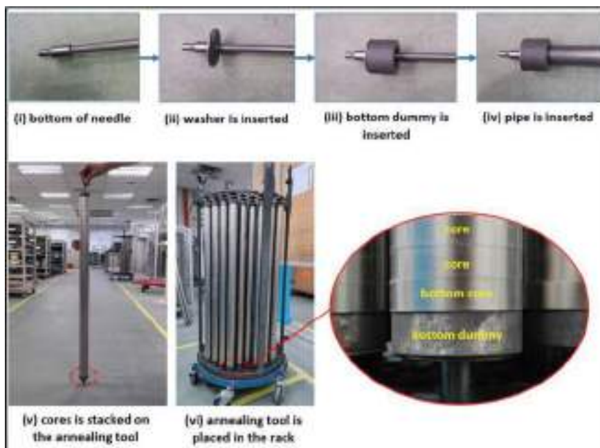
Fig. 1 The setup for annealing tools and the position of bottom core and dummy
